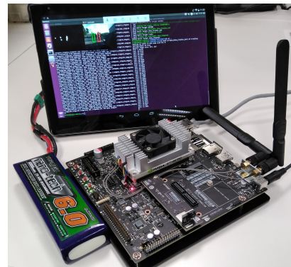
Fig. 1. Experimental set-up: live visual tracking is displayed on a tablet, which also controls the battery powered Jetson TX2 development kit used to capture and process the scene.
