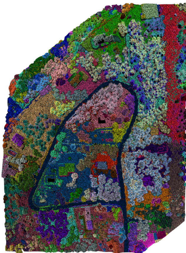
Fig. 4 Example of automatic segmentation using the graph-based approach.
