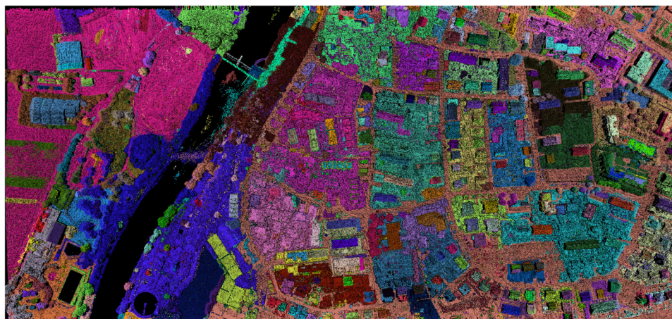
Fig. 12 Example of automatic segmentation using the single-graph-based approach (1645 groups).
