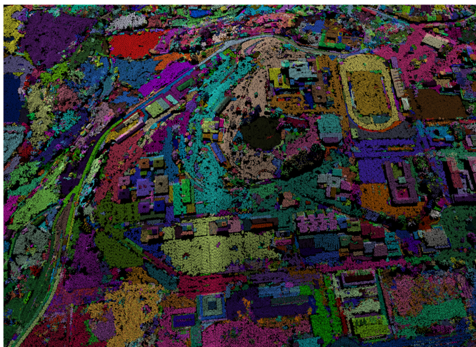
Fig. 13 Example of automatic segmentation on a dataset with very low-point density (0.5 points/m 2 ) using the interlaced-graph-based scheme.
