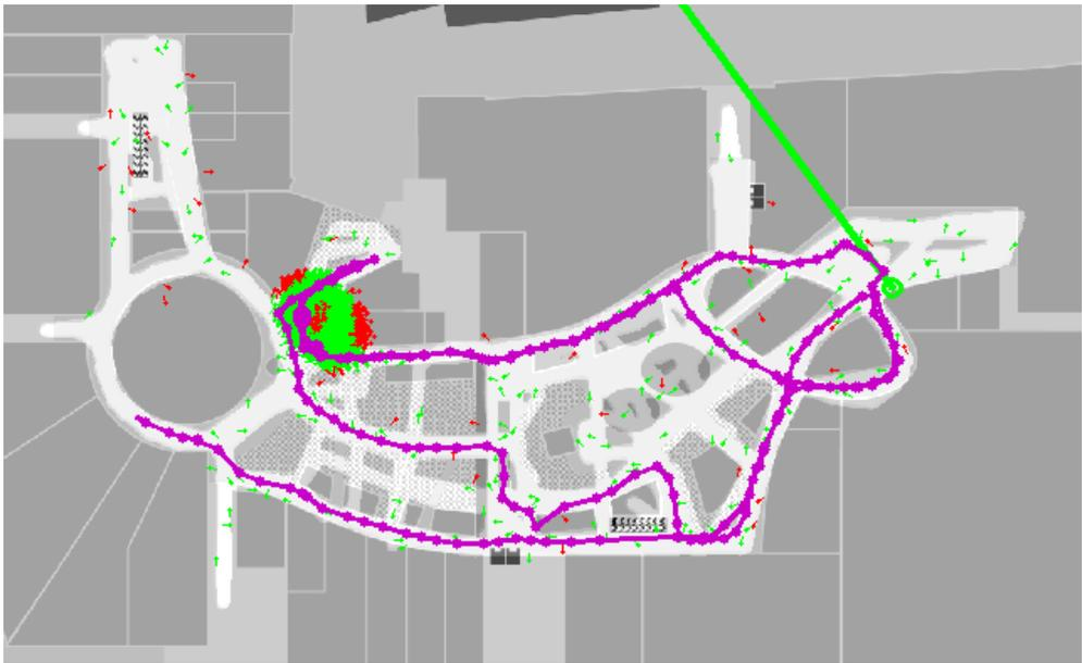
Figure 6.2: Example of a trajectory detected by the system. The purple dots and line represent the estimated positions and trajectory. The green area is a particle cloud around the user position at that moment of time.
