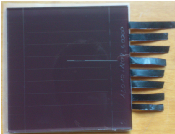
Figure 3.24: MM with every cell connected individually with a conducting adhesive side buss.
