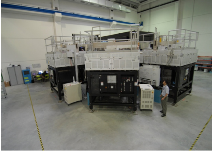
Figure 1.18: PECVD deposition cluster tool. It has an octagonal shape due to the fact that the seven deposition chambers and the load lock chamber, are all placed around a central transfer chamber.
