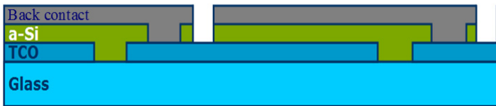
Figure 1.22: a-Si:H and back contact laser scribing step, P3 (cross section view).
