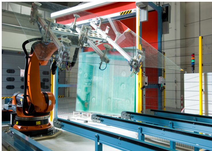
Figure 1.14: Kuka robot charging a front TCO-glass at the beginning of the production line.
