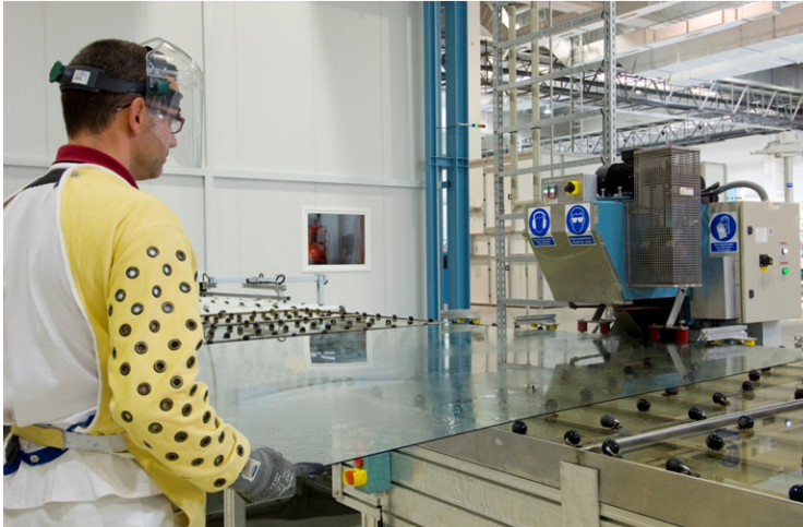
Figure 1.15: Operator seaming the front glass sheet with TCO layer.
