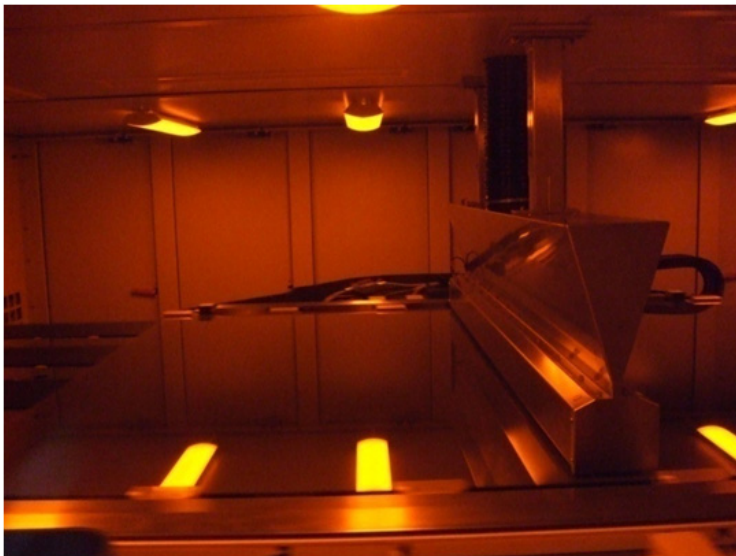
Figure 1.16: Laser tool picture. Panels are placed onto an air table.
