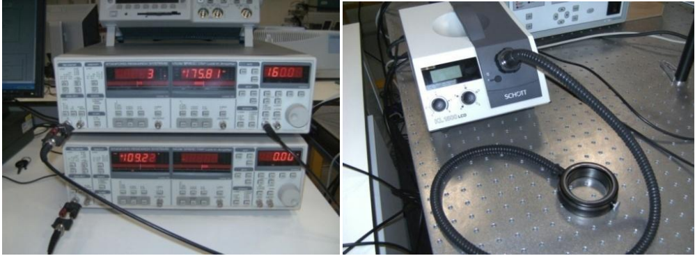
Figure 3.12: Two lock-in amplifiers (left) and cold light source with its illumination system (right).
