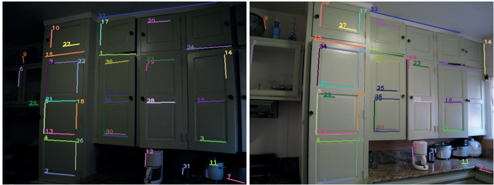
Figure 1.2: Example of line matching using the method described in this thesis, shown to highlight the difficulties due to line occlusions on a viewpoint change. Segment 6, colored in magenta, is mismatched due to occlusion by the limits of the frame. Segment 17, colored in cyan, is mismatched due occlusion by viewpoint change. Images from the dataset [74].
