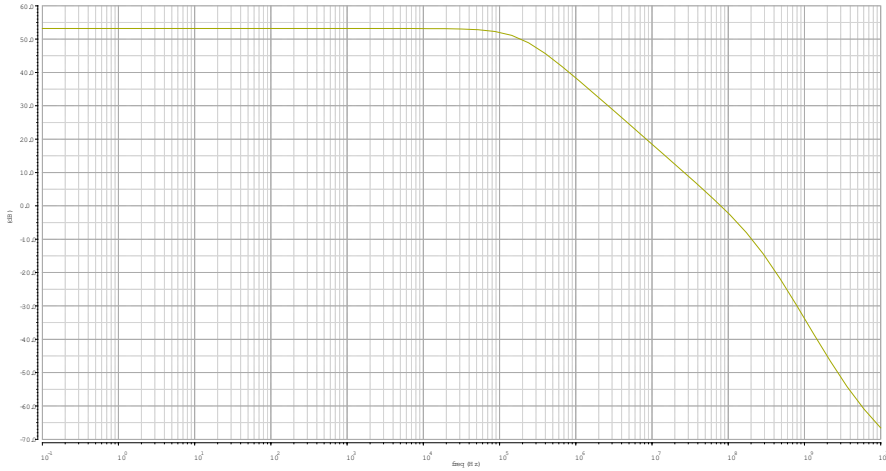
Figure 4.24: Bode plot of operational amplifiers OA5 and OA6.
