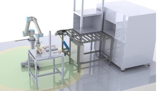
Design of a robotic cell with all the environment elements: furnace, molds...
