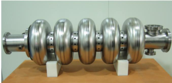
Two families of superconducting elliptical cavities, for  $\beta = 0.67$ , energy 216  $\rightarrow$  561 MeV and  $\beta = 0.86$ , energy 561  $\rightarrow$  2000 MeV. First high- $\beta$  prototype shown.
