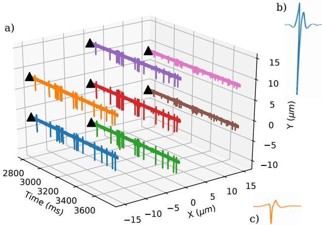
Fig. 5: a) Simulated recordings [20] for the probe topology. Here, an hexagonal probe is used. We only show 7 electrodes, in the same configuration as for our chip [21] [22]. Ground truth is available for classification performance estimation. b) and c) 2 different spike shapes extracted from the dataset.
