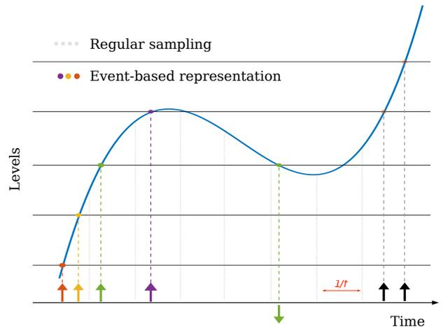
Fig. 1: Event generation. Each time the signal change, since the time of the last event (arrow), reaches a certain level, a new event is generated. The direction of this change, or polarity, is represented in the orientation of the arrow (up/down). For comparison, the grey dashed lines represent the standard, synchronous samples, uniformly distributed in time.
