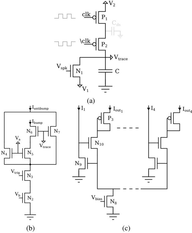
Fig. 3: Basic cells schematics: (a) Event trace circuitry; (b) Comparison circuitry [17]; (c) Basic WTA circuit [18], two inputs are shown. See text for details.
