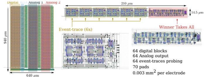
Fig. 6: Layout of the hereby described chip. The core is composed of  $3 \times 64$  basic blocks (6 decaying units, 4 template matching and a WTA). The outputs are multiplexed to spare output pads. The core occupies a space of  $640 \times 940 \mu m$ , each individual block being  $14.5 \times 210 \mu m$ .
