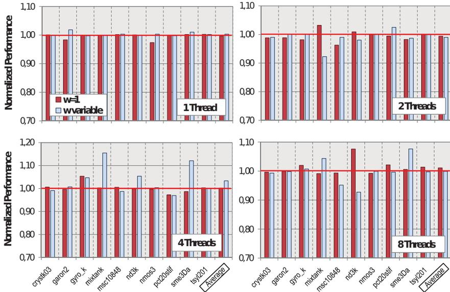
**Figure 4.9:** Normalised SpMV performance obtained by the reorderings generated using the locality optimisation technique and the information provided by the hardware-counter sampled matrices for windows of size  $w = 1$  and variable size.
