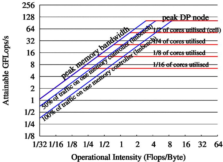
Figure 2.16: Ceilings added to the FINISTERRAE Roofline Model.
