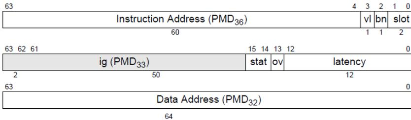
Figure 2.7: Data Event Address Register Format ( $PMD_{32,33,36}$ ).
