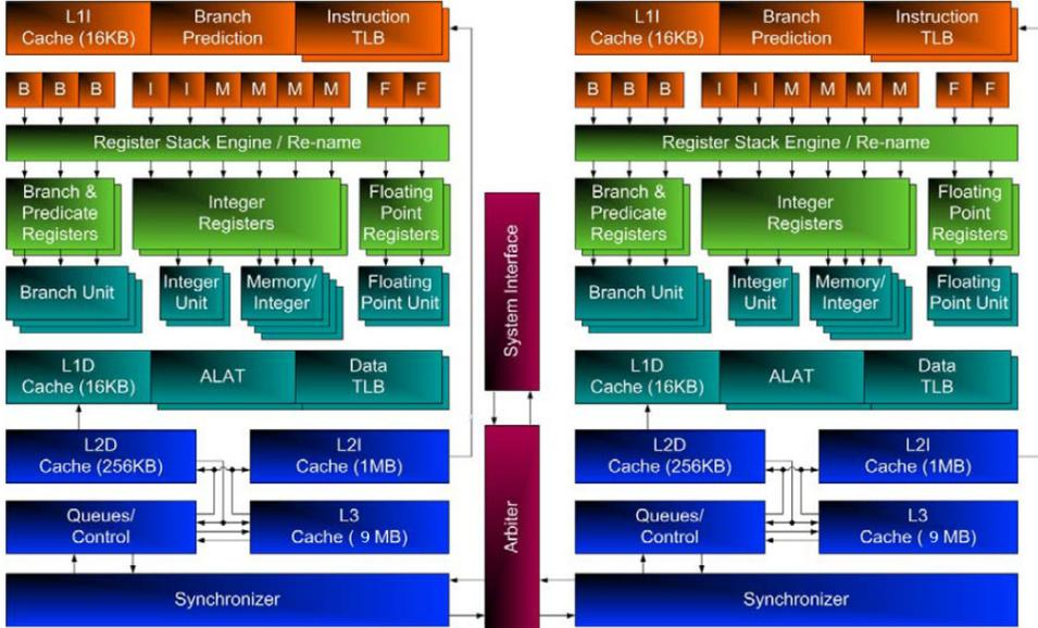
Figure 2.4: 1.6 Ghz Dual-Core Intel Itanium2 Montvale (9140N) architecture [2].
