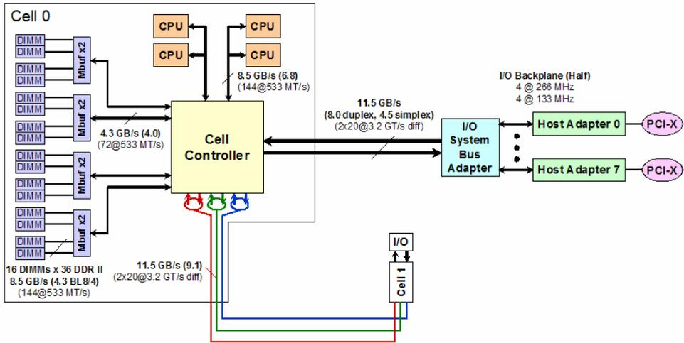
Figure 2.1: HP Integrity rx7640 node (taken from [1]).
