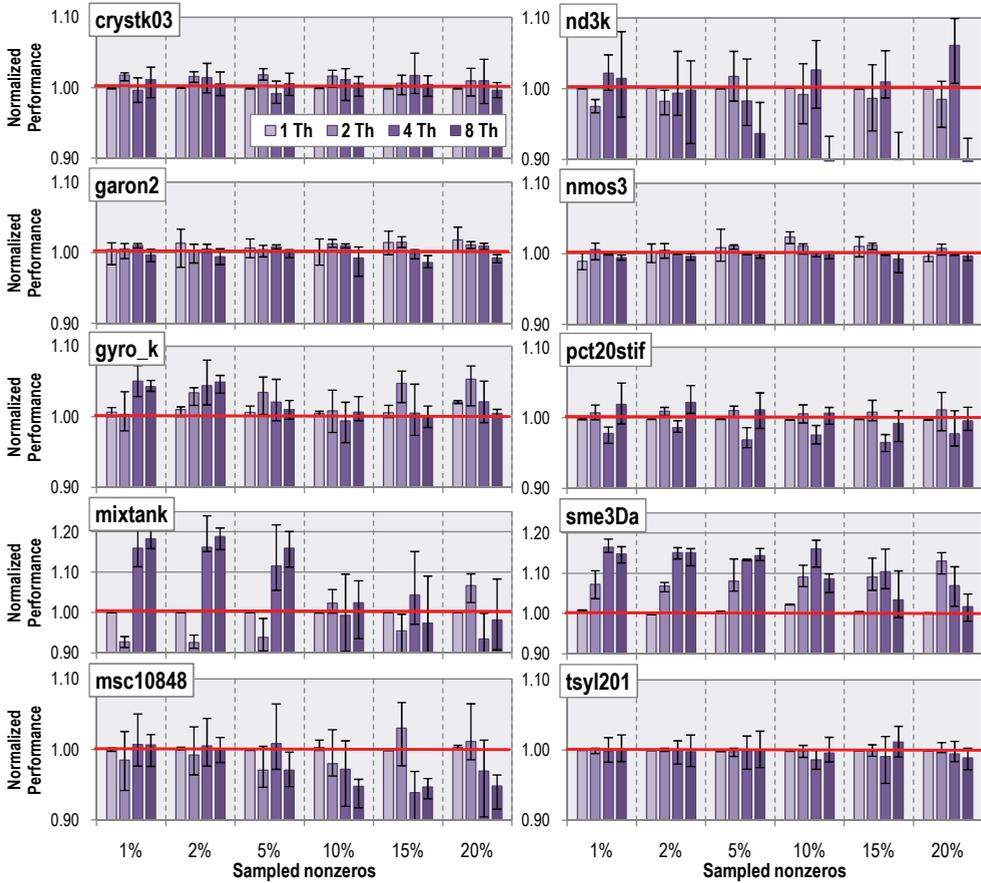
**Figure 4.5:** Normalised SpMV performance obtained by the reorderings generated using the locality optimisation technique ( $w = \text{variable}$ ) and the information provided by the randomly sampled matrices on the Itanium2 platform.
