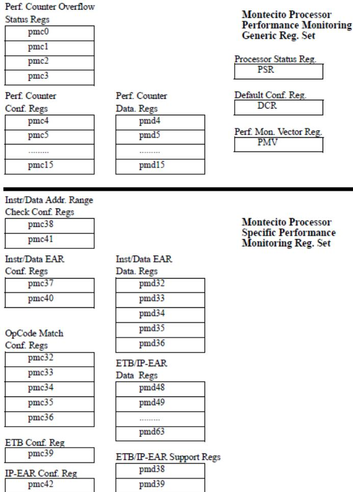
**Figure 2.5:** Montecito/Montvale Processor Performance Monitor Register Set [2].
