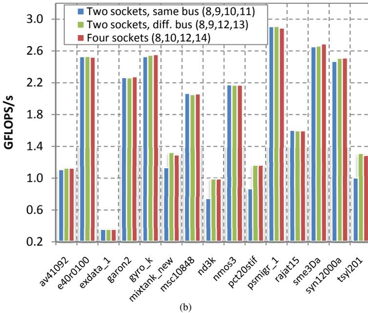
Figure 2.13: Influence of the thread allocation on a rx7640 node: using two (a) and four threads (b).
