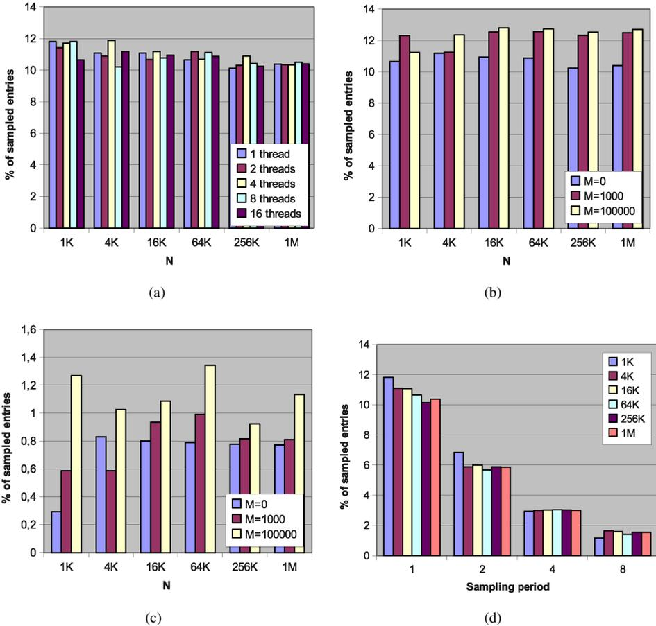
**Figure 3.5:** Ratio between the number of sampled entries of vector  $X$  and its size. (a): for different values of  $N$  and number of threads;  $X$  is a vector of floats. (b): for different values of  $N$  and  $M$ ;  $X$  is a vector of floats. (c): for different values of  $N$  and  $M$ ;  $X$  is a vector of integers. (d): for different values of  $N$  and the sampling period;  $X$  is a vector of floats.
