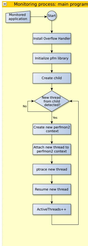
**Figure 5.4:** Flow diagram from the main function of the monitoring tool.
