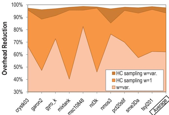
**Figure 4.10:** Overhead reduction of the locality optimisation technique using as a reference the time required to perform the reordering using windows of fixed size  $w = 1$  and the original (non-sampled) matrices.
