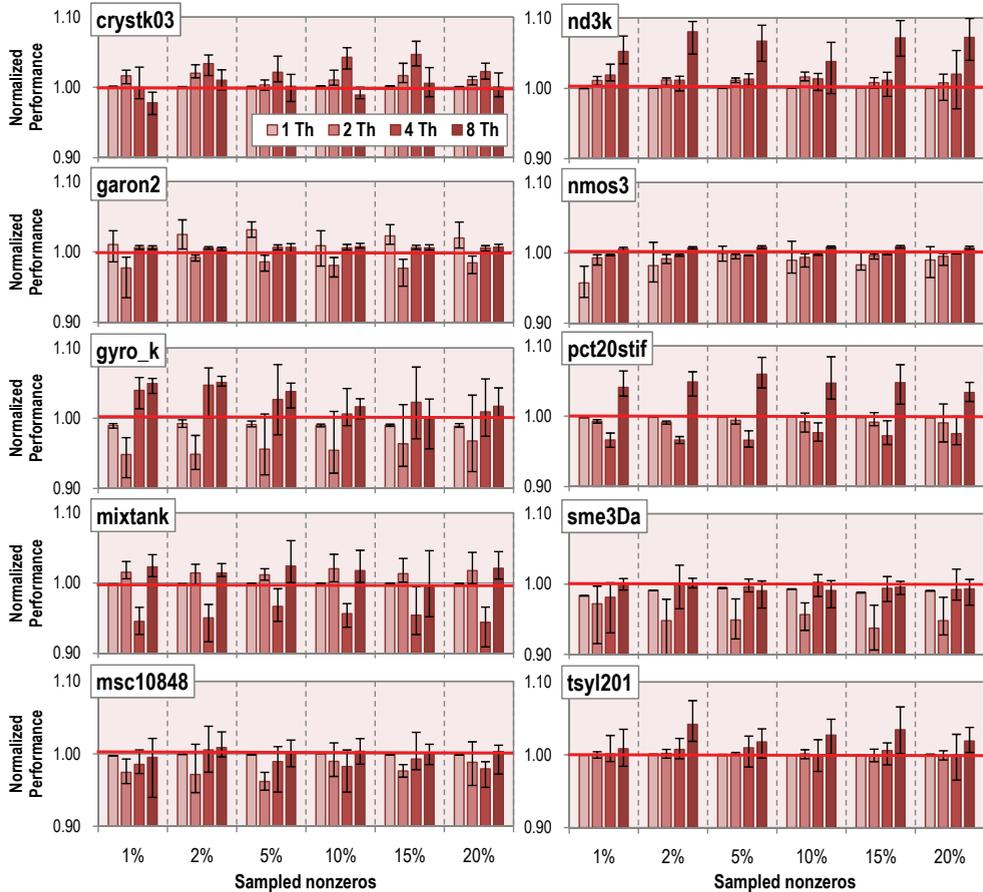
**Figure 4.4:** Normalised SpMV performance obtained by the reorderings generated using the locality optimisation technique ( $w = 1$ ) and the information provided by the randomly sampled matrices on the Itanium2 platform.
